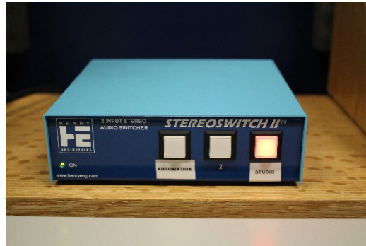
Fig.4 On-Air Switch (red button lit), studio LIVE TO AIR
