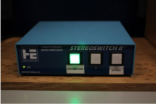
Fig.3 On-Air switch, normal operation, automation on-line, studio pre-recording shows
